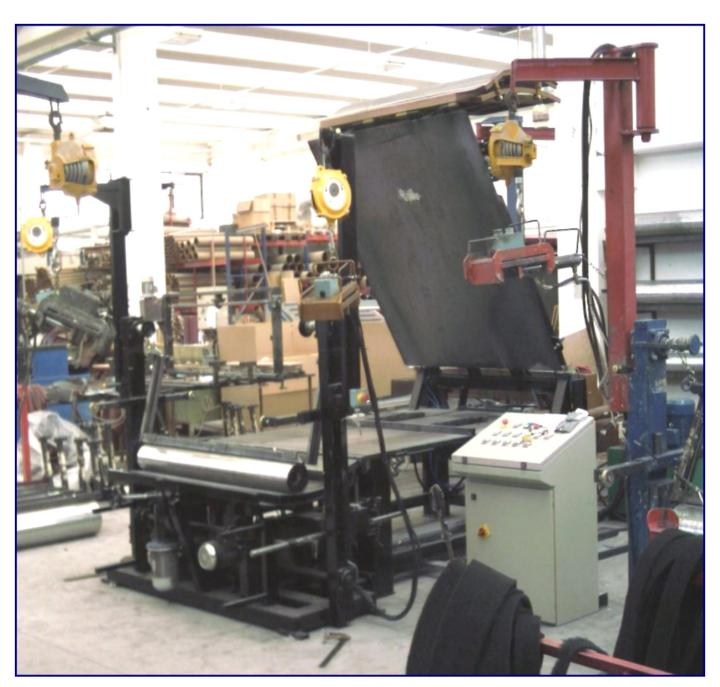
This is a machine for the production of abrasive rollers; maximum working sizes are 500mm diameter and 1500mm standard length. A hydraulic cylinder presses the material and two operators put it into the moulds.
